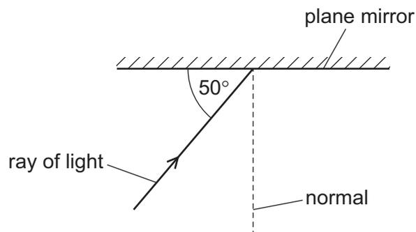
What is the angle of reflection of the ray when it is reflected from the mirror?
