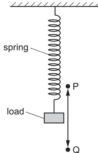
The load is pulled down and then released so that it oscillates between point P (highest point) and point Q (lowest point).
